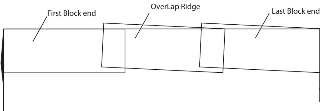
By installing a dentil slip (packing slate) all ridge tiles will follow the same line.
