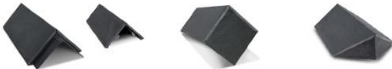
*Natural 12mm thick Brazilian slate, bonded to a Glass Reinforced Polyester (GRP) substrate, with aluminium rivets for secondary mechanical fixing. Features built-in free air ventilation strip and patented clip and connector system for easy fixing and waterproofing. For use as a preformed angular dry-fix hip or ridge tile. Fixing holes pre-drilled and all fixings supplied.*
