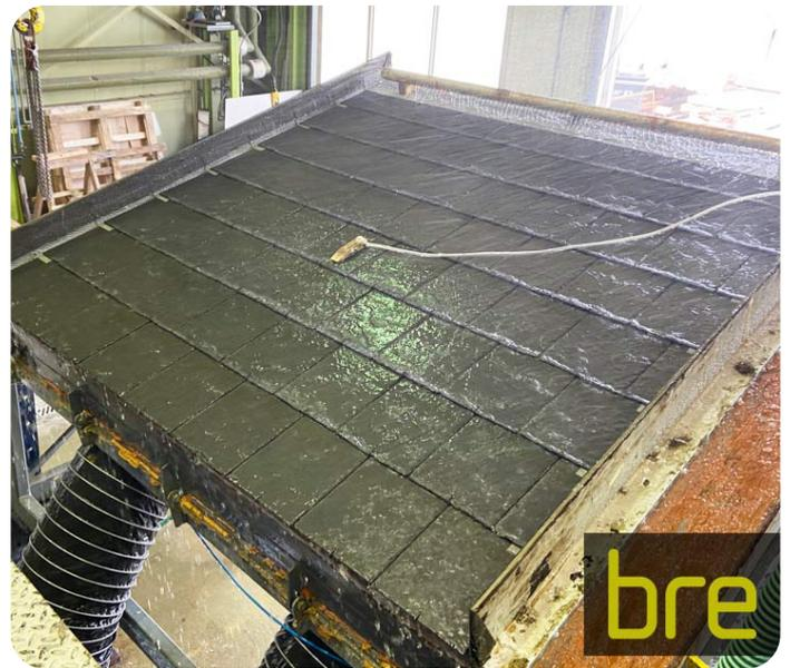
**The Mayan ArmouredSlate roofing system dramatically improves the overall performance of a natural slate roof. Our system is watertight and durable down to 10 degrees.**
