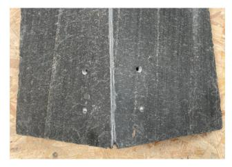
**Block ends and ridge caps are supplied unholed** because the position of the drill holes are dependent upon individual roof applications. Cut tiles also require drilling.
