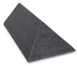
Natural Spanish slates, bonded to a Glass Reinforced Polyester (GRP) substrate, with aluminium rivets for secondary mechanical fixing. For use as a preformed, angular, dry hip or ridge tile. Fixing holes pre-drilled and fixings supplied.
